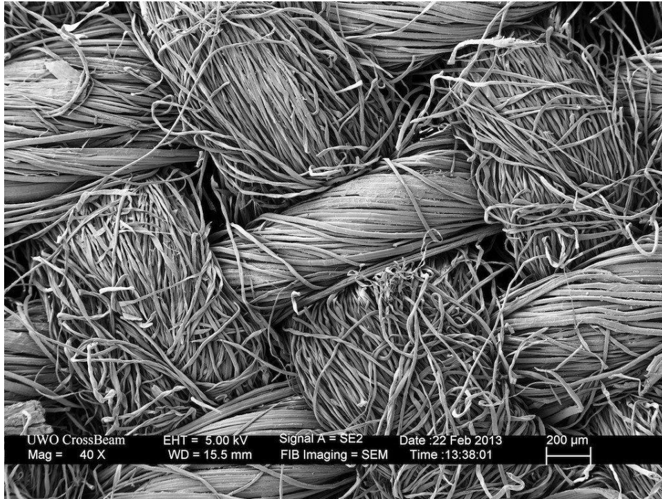
Cotton cloth photo at 40x magnification
